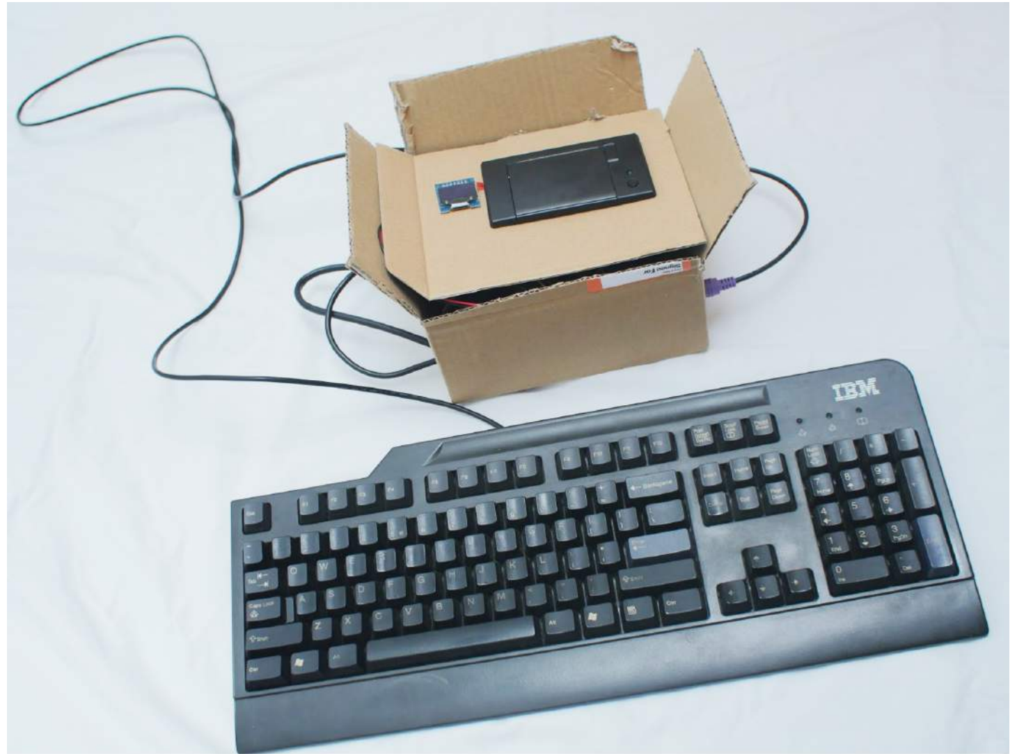
Skjøtt | portable, battery-operated receipt printer typewriter
